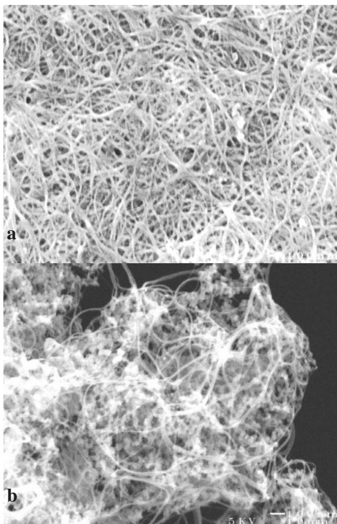
**Fig. 3.** **a** SEM image of the surface of bucky paper after the first cross-flow filtration step. **b** SEM image of the 4" material shown in **a** prior to purification (raw material)
