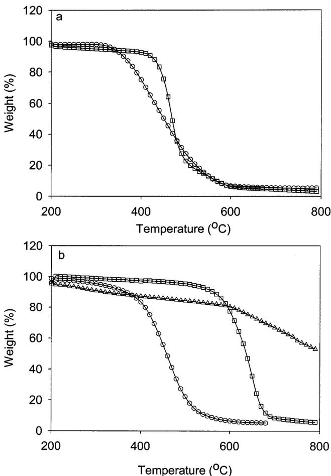
**Fig. 10.** **a** TGA data in air of raw SWNT material ( $\circ$ ) and the same material which was vacuum baked at 1200 °C for 14 h ( $\square$ ). **b** TGA data in air of purified SWNT material which has ( $\circ$ ) and has not ( $\square$ ) been vacuum baked as above. The curve marked ( $\Delta$ ) is unbacked, purified material run in a 0.1% oxygen (argon balance) atmosphere. See text for discussion
