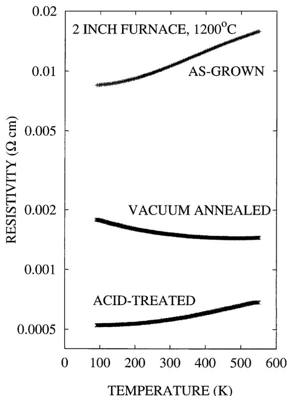
**Fig. 11.** Four-probe resistivity vs. temperature for 2" material. The acid purification results in a  $\approx 25$ -fold reduction in  $\rho$  with little change in temperature dependence. Vacuum annealing increases  $\rho$  somewhat and the  $T$  dependence changes from metallic to non-metallic (see text)
