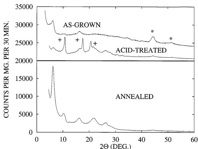
**Fig. 6.** Raw X-ray data for 2" SWNT material. TOP (zero shifted to 20 000 for clarity): as-grown and acid-treated material. (\*) indicate peaks from Ni/Co catalyst and (+) are indexable as fcc  $C_{60}$ . BOTTOM: after final vacuum anneal
