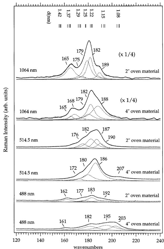
**Fig. 9.** Raman spectra in the vicinity of the radial mode frequency for the 2" and 4" material collected using the indicated excitation frequencies. Vertical bars represent the positions of the calculated radial mode frequency for zigzag, armchair and chiral SWNTs. Individual Lorentzians are also indicated in the figure (see text)
