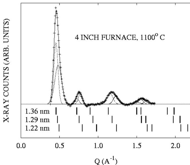
**Fig. 8.** Similar to Fig. 7 for 4" material. Note the overall shift to smaller diameters, which we associate with the lower growth temperature (1100 °C vs. 1200 °C in Fig. 7). Note also a possibly broader diameter distribution. The fit is truncated at  $1.7 \text{ \AA}^{-1}$  due to the presence of graphite (002) at  $1.86 \text{ \AA}^{-1}$
