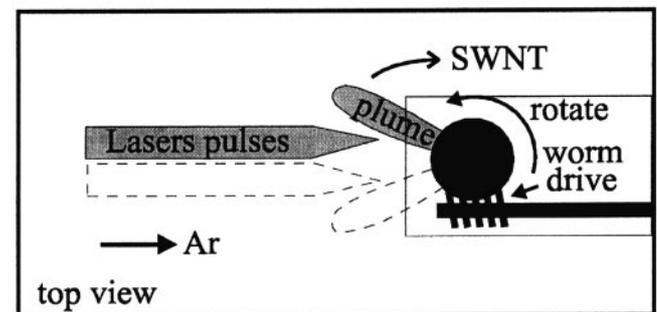
**Fig. 2.** The configuration in the 4" system. The target rotates about its vertical axis. The laser beams are swept up and down one side of the target (*side view*) for several minutes before periodically being shifted to the other side of the target (*top view*), where they again sweep up and down the side of the target
