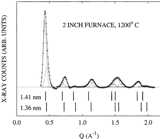
**Fig. 7.** Gaussian fits to background-subtracted data from annealed 2" material. (++++) are the data; the solid line is the composite fit and the dashed lines are Gaussians with fixed  $0.06 \text{\AA}^{-1}$  FWHM. Tick marks below indicate the expected positions from triangular lattices of 1.41-nm and 1.36-nm-diameter tubes, accounting for particle size broadening and the circular form factor
