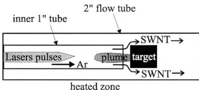
**Fig. 1.** The configuration in the 2" system capable of giving a fractional SWNT yield comparable to that of the original 1" system but at  $\approx 1$  g/day production rate
