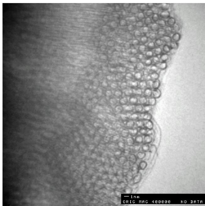
**Fig. 4.** Cross-sectional view of a SWNT rope permitting direct measurement of nanotube diameters. Measurements were only made on those tubes for which the tube wall was unambiguously distinct in the image
